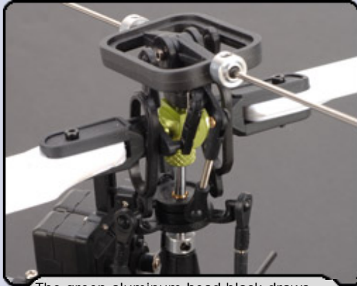
The green aluminum head block draws attention to the NR3D's CCPM system, a fairly standard 3-servo setup that works well.
