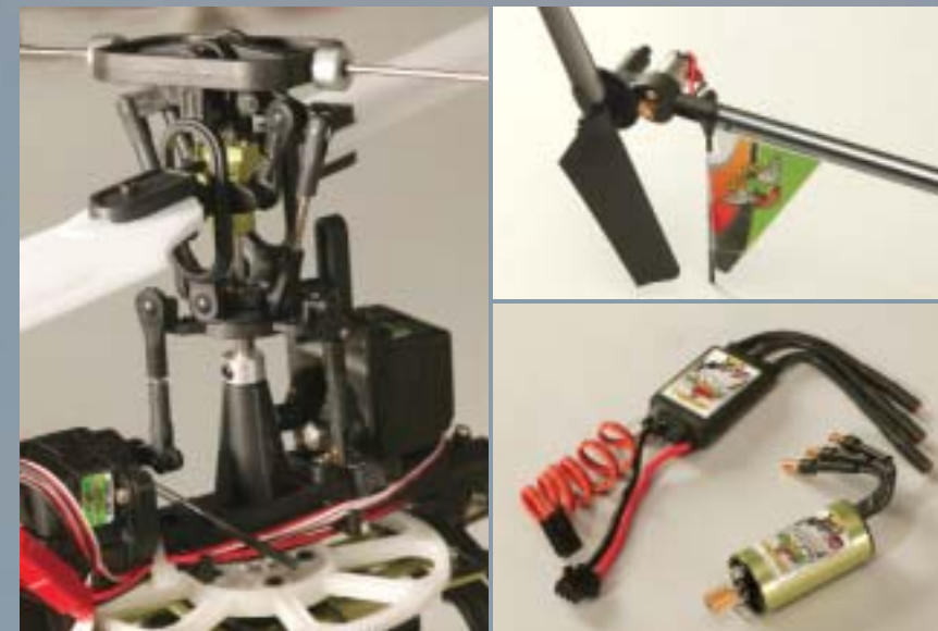
Left: Direct servo linkages ensure precise CCPM control. Top right: The separate tail rotor motor offers easy setup and maintenance, and solid response. Bottom right: For maximum performance, Venom offers this brushless motor specifically matched to the Night Ranger 3D.
