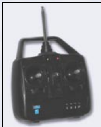
Figure 6 - The Radio Transmitter
