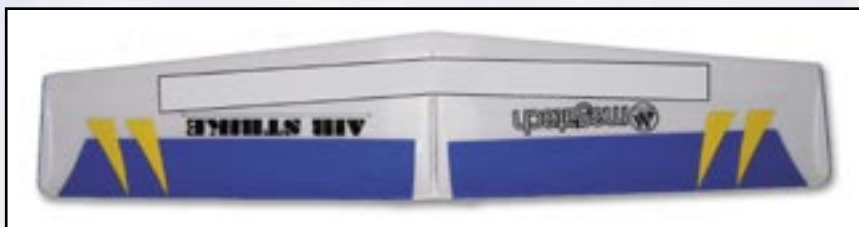
Figure 3 - Place PVC tape along bottom of wing as shown.
